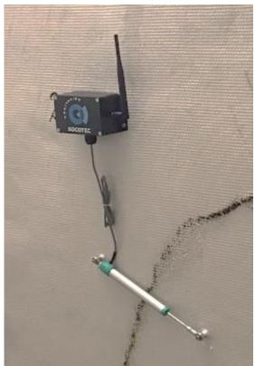
Figure 12: Photo of a NodeLog installation with 100mm GEFRAN transducer
